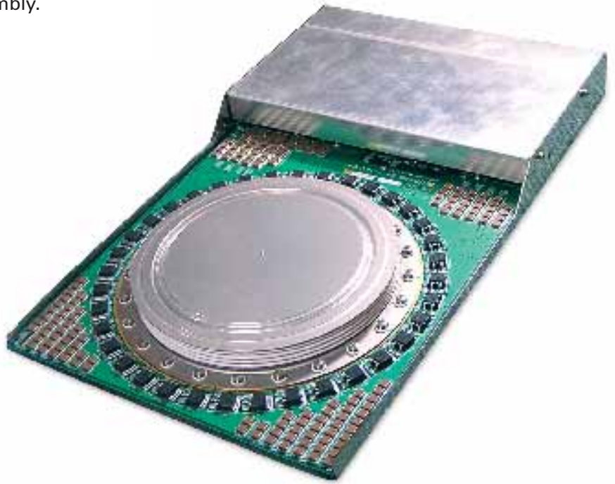
GCT Assembly showing firing circuits and control board, four per half-module
